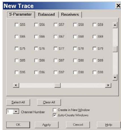
Figure 32 14-Port New Trace Measure (S55 - S99)
