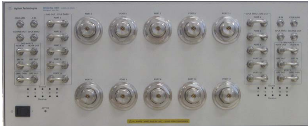
Figure 3 Front Panel (Multiport Test Set)
