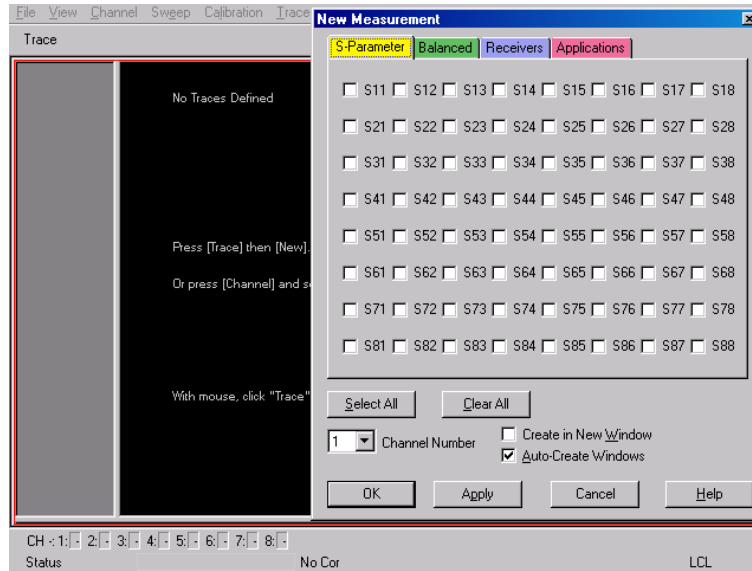
Figure 20 12-Port New Trace Measure (S11 - S88)
