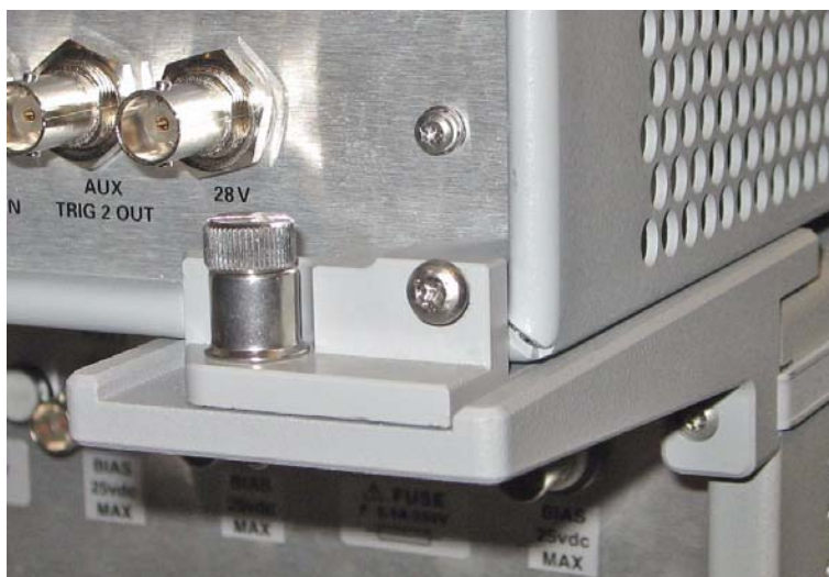
Figure 10 Locking Feet Screws
